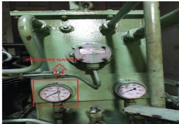
***Pressure gauge hydraulic steering gear***
