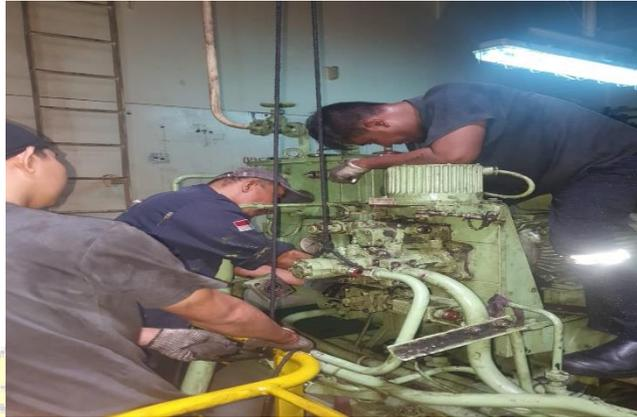
**Proses *overhaul* hydraulic pump steering gear**
