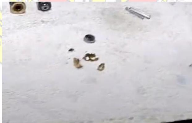
**Kerusakan Pada *piston* hydraulic pump steering gear no. 2**
