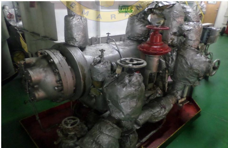
Gambar Furnace Condenser MV. Kartini Samudra
