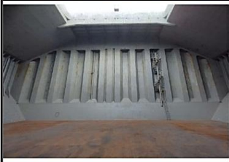
1. Forward Transverse bulkhead
