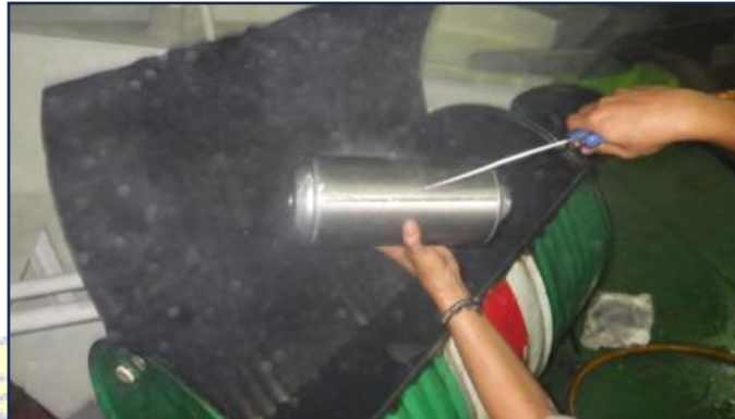
Gambar 4.8 pembersihan filter lo gearbox
