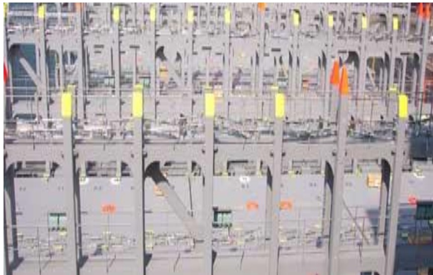
Gambar Lam.1 Lashing Bridge dan Hatch Cover.
