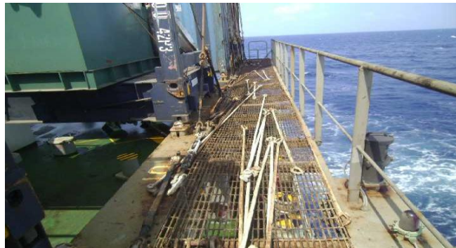
Gambar Lam.13 Lashing Gears berserakan di Lashing Bridge .
