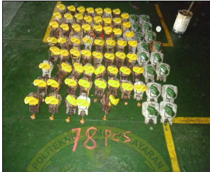
Gambar Lam.8 Perawatan Twist-lock .
