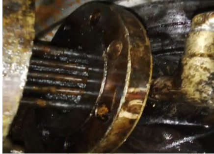
Gambar 4. Kotornya Electric Heater
