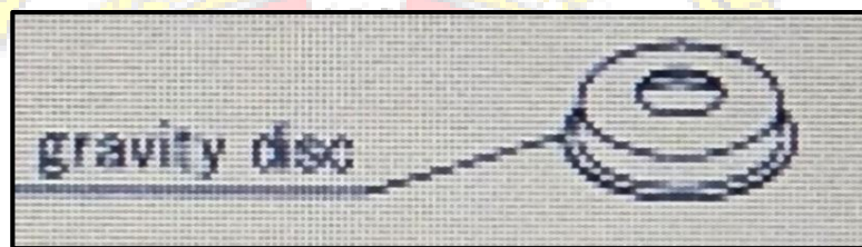
Gambar 2. 15 Gravity disc Sumber : Manual book purifier
