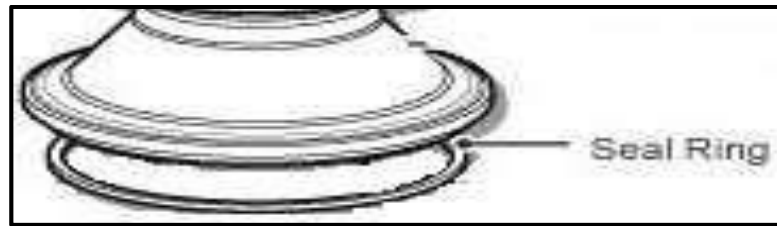
Gambar 2. 11 Main seal ring Sumber : Manual book purifier
