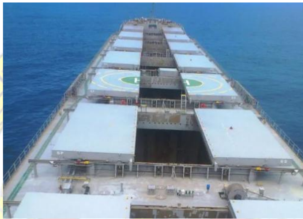
Gambar 2. 2 Hatch cover tipe geser
