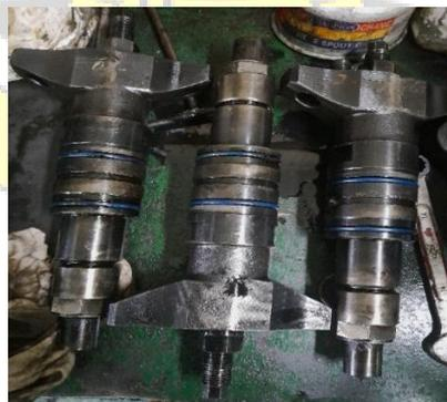
Gambar 2.3 *Injector DG*
