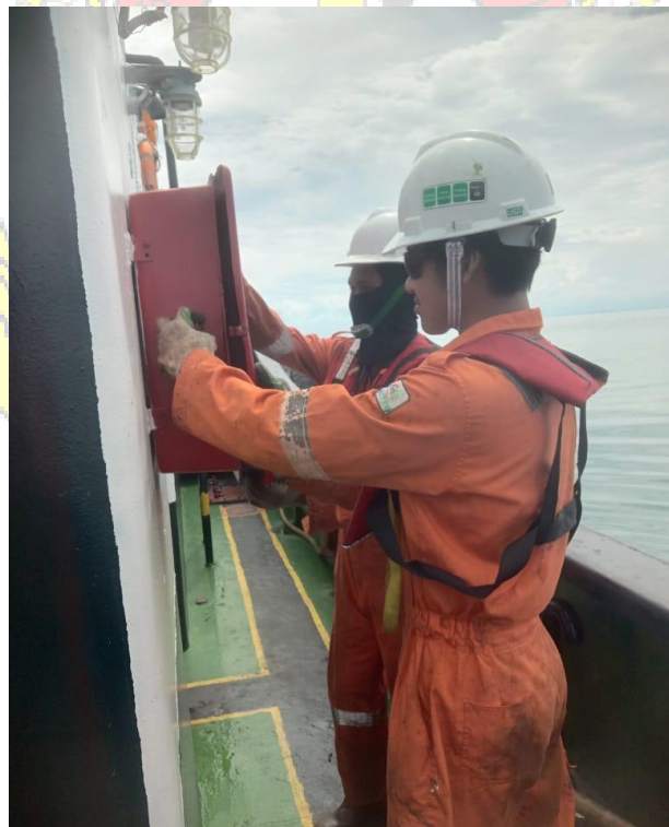
Inspection firebox tugboat PT. Kartika Samudra Adijaya
