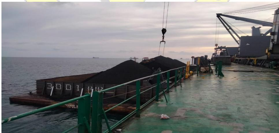
**Gambar 2. 1 Proses Transshipment Dari Tongkang Ke Vessel**
