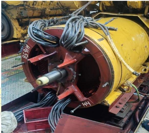
Gambar 2. 2 *Alternator Diesel Generator*
