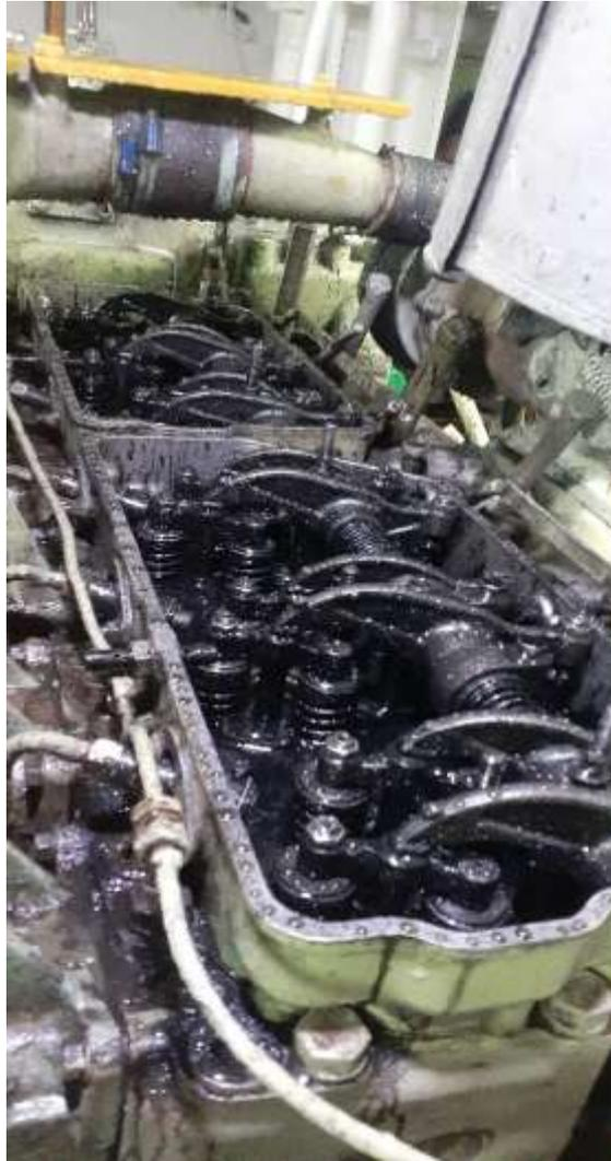
**LAMPIRAN VI****Proses Penggantian *Exhaust Manifold* dan *Cylinder Head***
