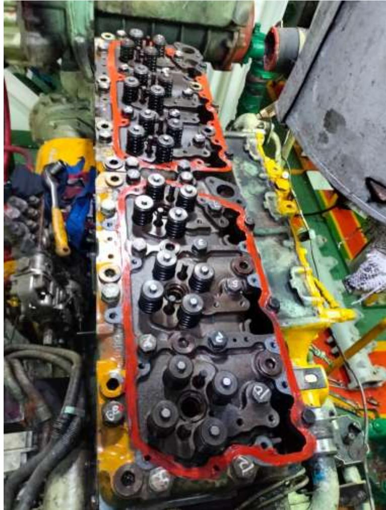
**LAMPIRAN VIII****Kondisi Setelah Penggantian *Exhaust Manifold***
