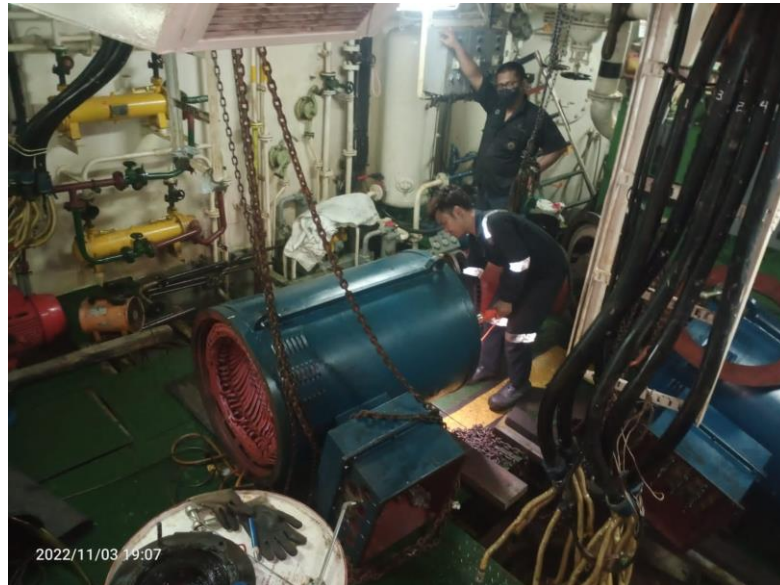
Gambar 1. Proses overhaul bow thruster di galangan kapal
