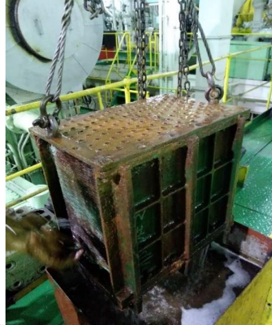
Pembersihan tube sea water side
