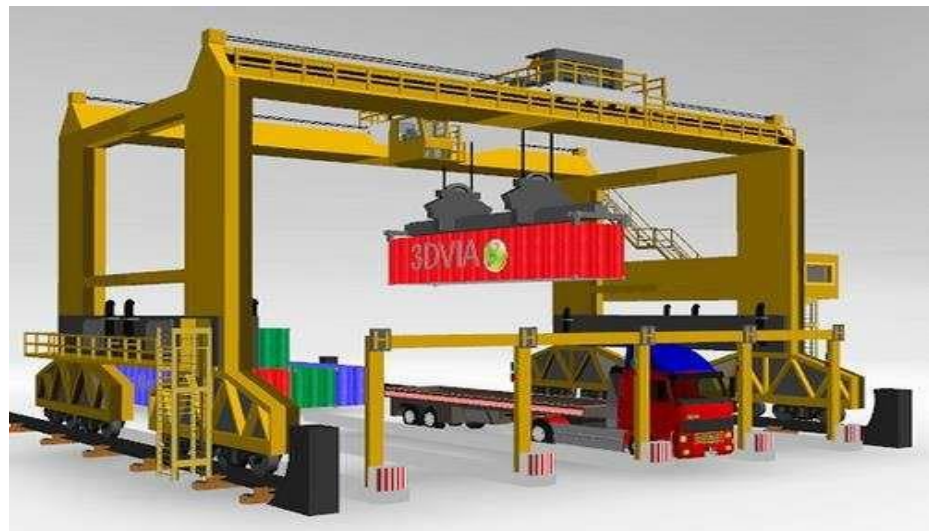
Rail Mounted Gantry Crane (RMGC)
