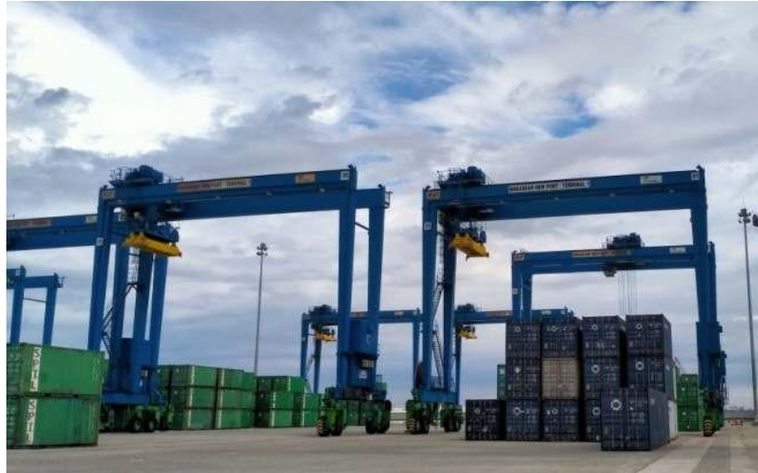
Rubber Tyred Gantry (RTG) Crane
