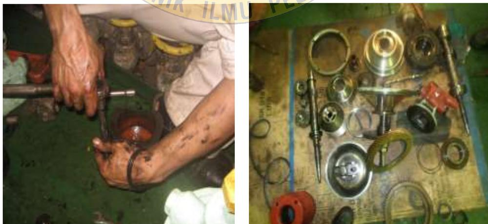
Gambar 4.9 Proses *Overhaul LO Purifier*
