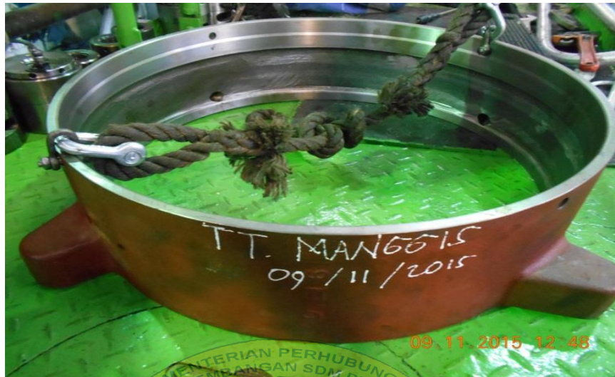
Gambar 2.2 Jacket cooling bagian cylinder cover main engine .
