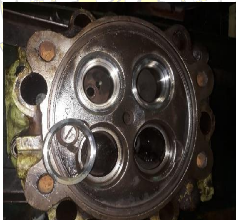
Pemasangan seating valve
