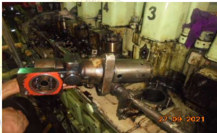
Gambar 2. 5 Fuel Injection Pump Sumber: Dokumen Penelitian Di Olah, 2021
