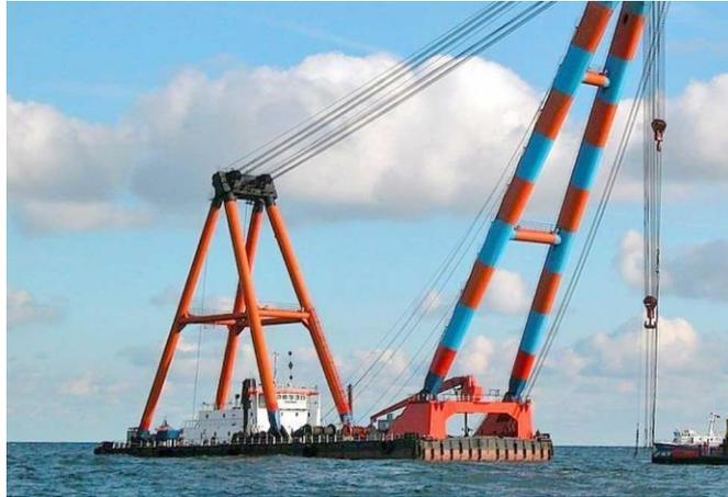
Gambar 1.2 Contoh *Crane* ponton
