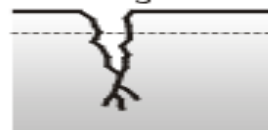
Gambar 2.7 mekanisme Stress Corrosion Cracking
