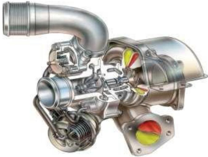
Gambar 2.11 *variable scroll turbocharger*
