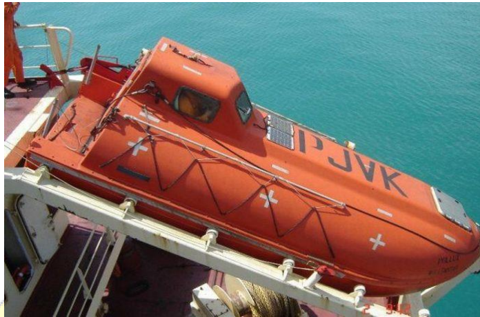
Gambar 2.3 Free Fall Lifeboat Sumber: https://acidcow.com
