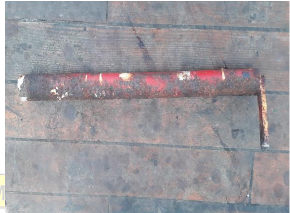
Gambar 2: As Lock Roda Sekoci
