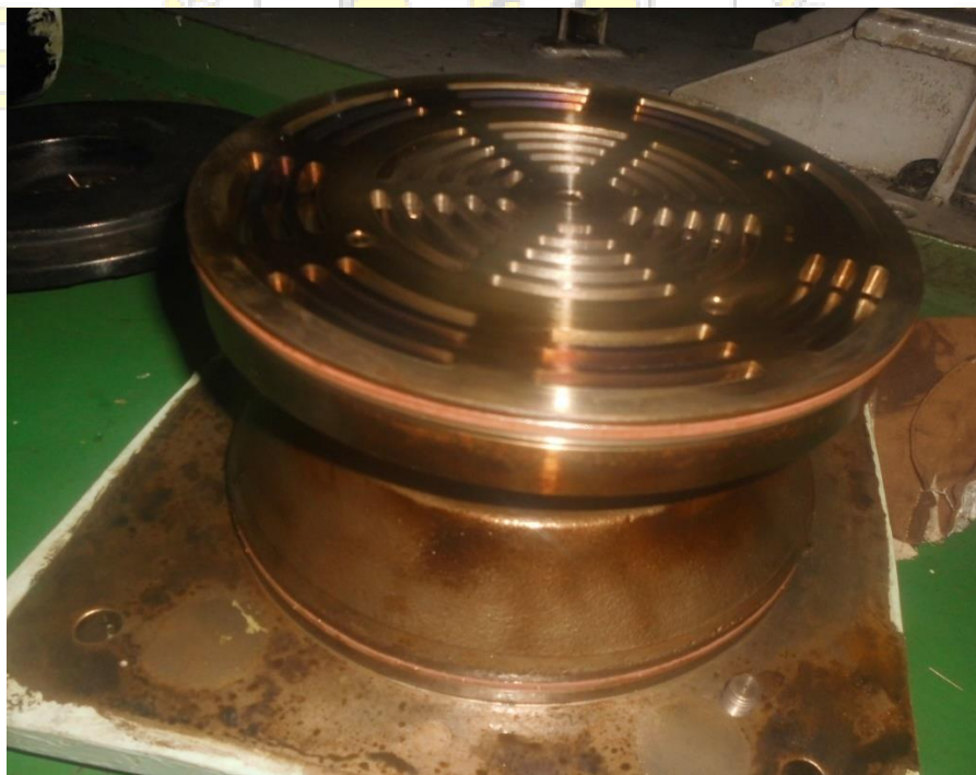
Gambar Pemasangan New Spare Part First Stage Valve
