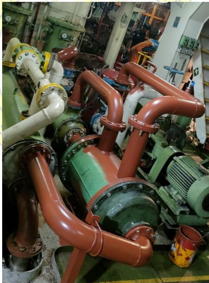
Gambar pengecatan dasar fresh water cooler tambahan.
