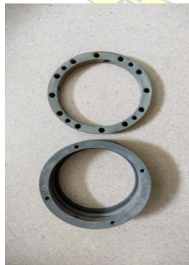
Mechanical seal lama/sudah dipakai
