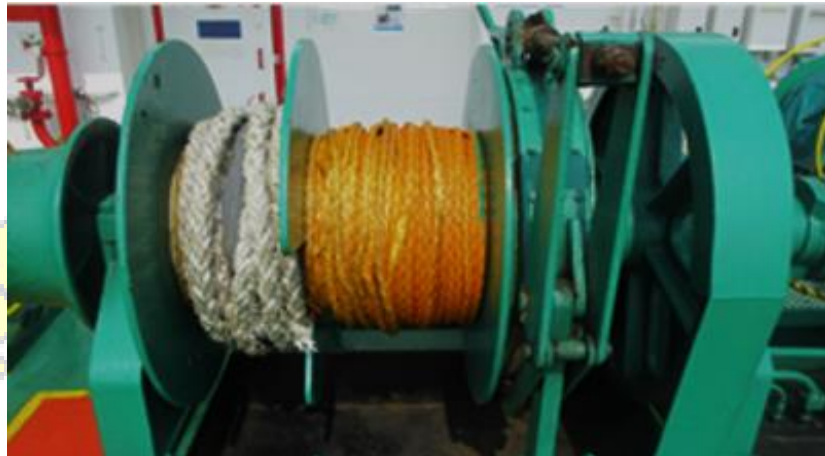
Gambar 2.13 Mooring Winch (Sumber : Mooring System Management Plan Lines Management Plan 2021 format PIS rev August 2021 )
