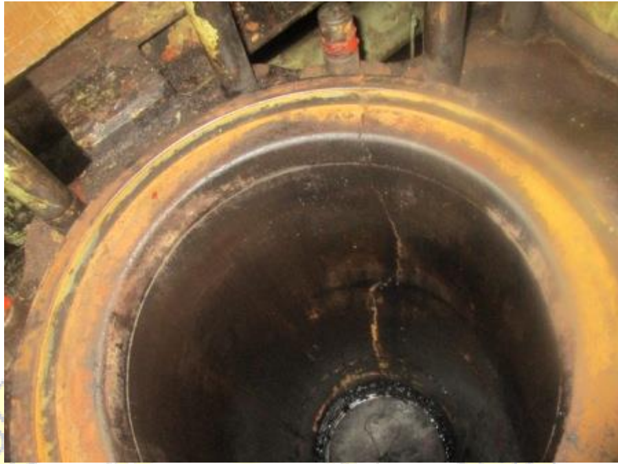
Gambar Retaknya Cylinder Liner Main Engine
