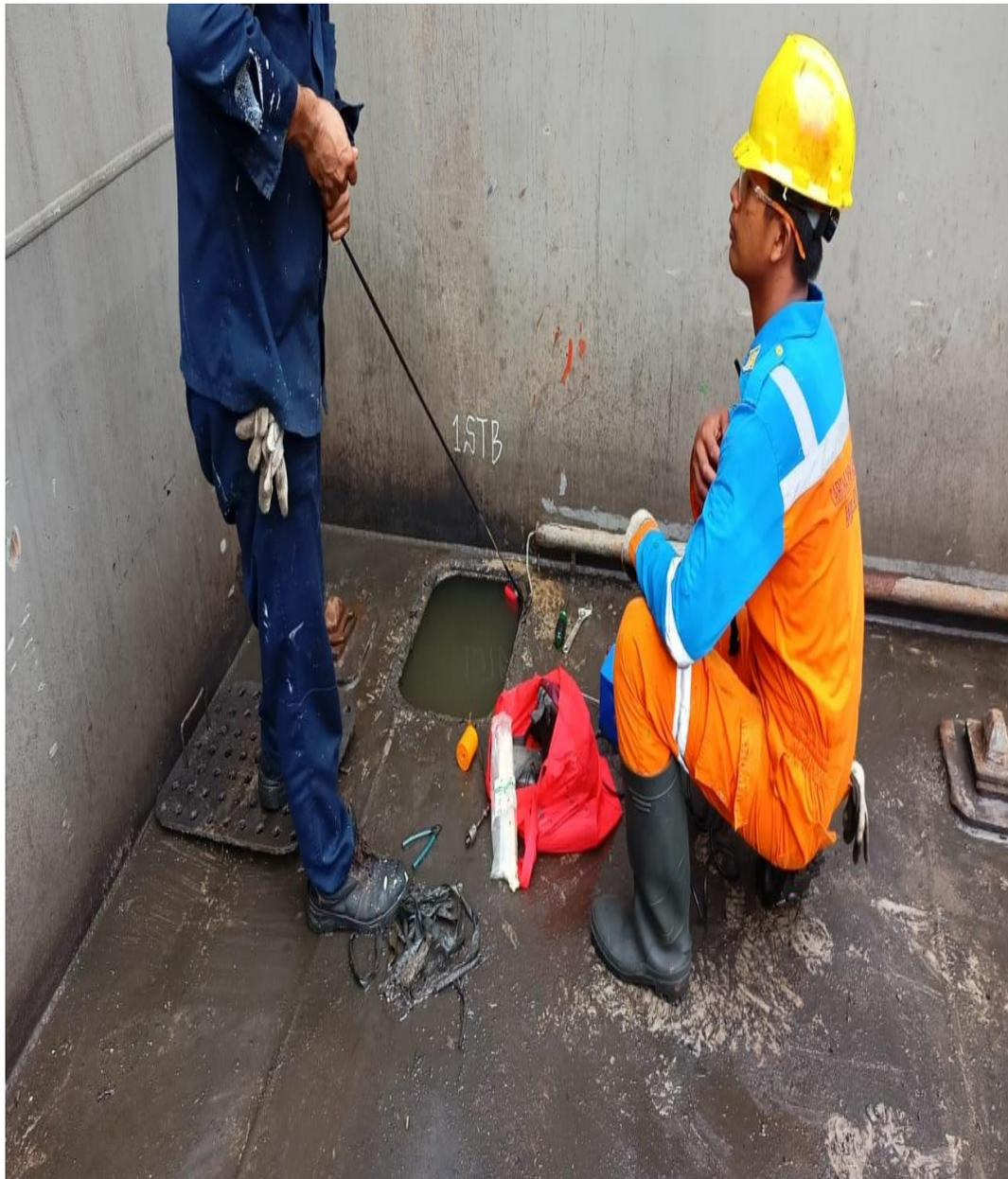
**LAMPIRAN 5*****TEST FLOATING SWITCH SENSOR OLEH ELECTRICIAN***
