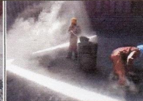
Cargo residue being swept by fine sweeping & collected.
