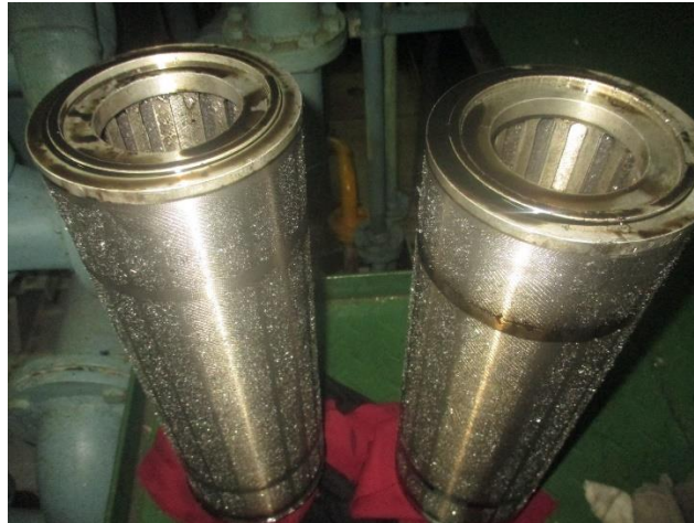
Kondisi L.O filter Aux. Engine kotor
