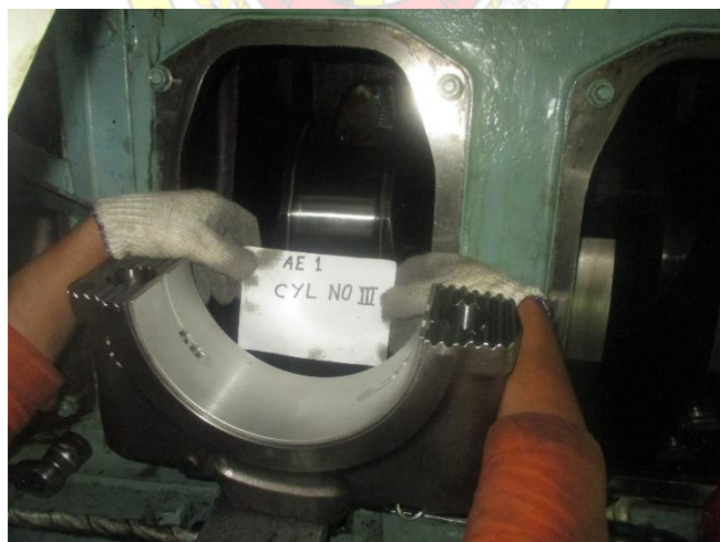
Pengantian crankpin bearing Aux. Engine
