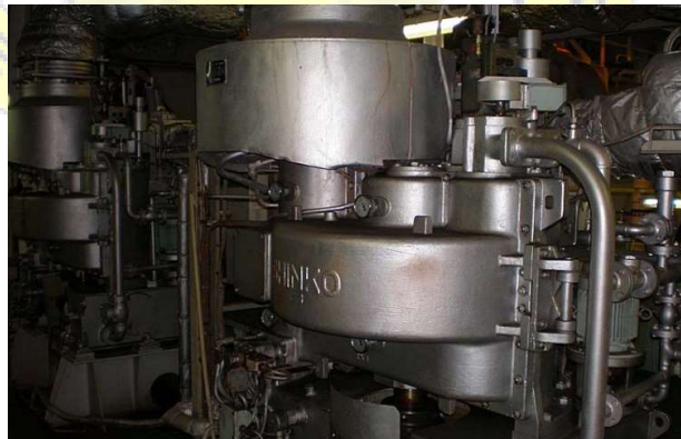
Gambar 2.1 Cargo oil pump turbine MT. Nusa Merdeka
