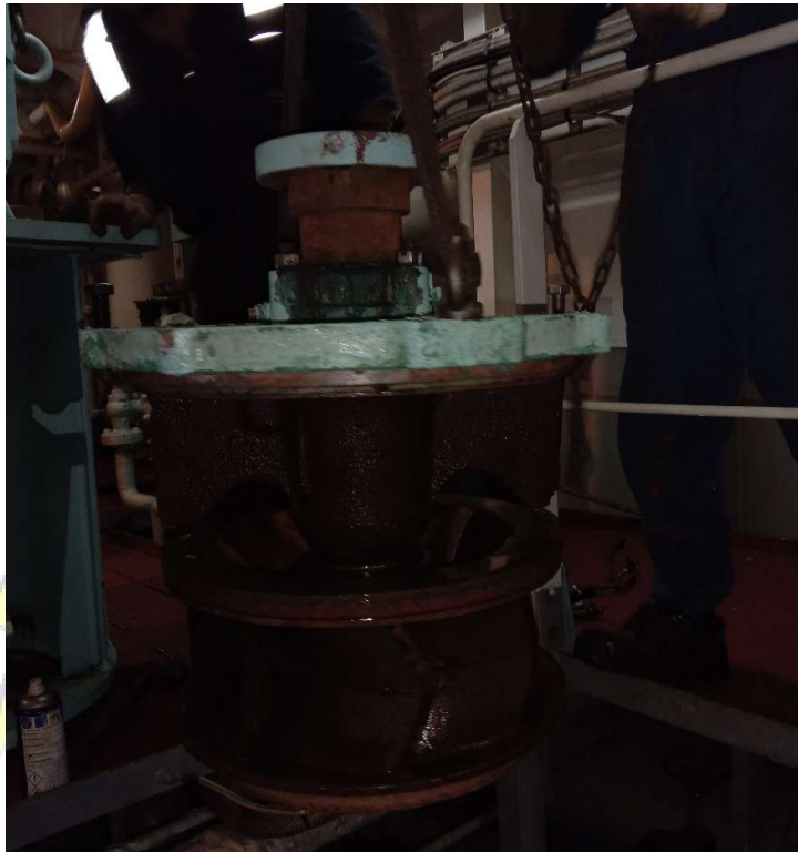
Lampiran 8. Overhaul Cargo Oil Pump Turbine
