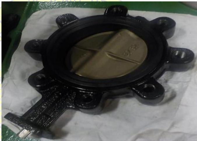
Gambar 2.1 Valve (*butterfly valve*)
