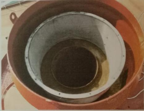
Mast riser Flame screen and Cleaned:
