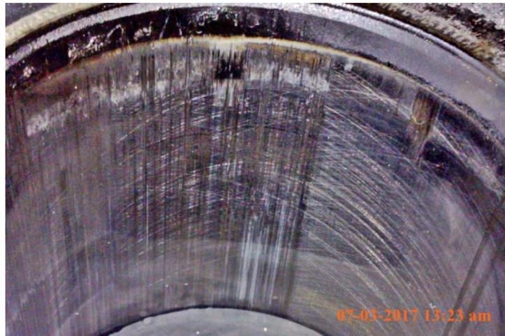
**Gambar 2.2 Liner Silinder Mengalami Abrasive Wear**
